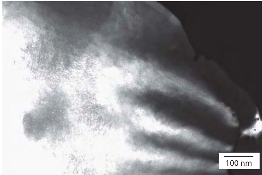
Figure 3.9: Dark field image of the \text{LAO}(001) surface after a 3 hour anneal at 800^\circ\text{C} . Preliminary faceting is visible in the image. As the anneal time increases larger facets with fewer defects result.
