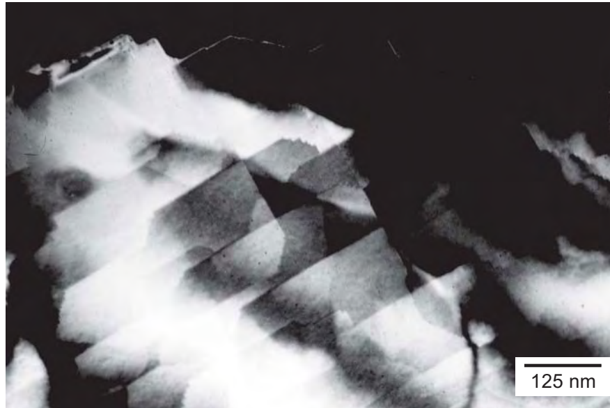
Figure 3.11: Dark field image of the (\sqrt{5} \times \sqrt{5})R26.6^\circ surface on LAO after a 3 hour anneal ( 1100^\circ\text{C} ). The formation of \langle 100 \rangle facets, with respect to the cubic face, occur at this temperature and can be seen in the image. Small rectangular features are discernible near the edge of the sample. These features do not show any strain contrast in the image which suggests they are not particles or trapped gas. Similar voids have been observed on other perovskite materials, like \text{SrTiO}_3 . This reconstruction is extremely reproducible and has been shown to be air stable for several months.
