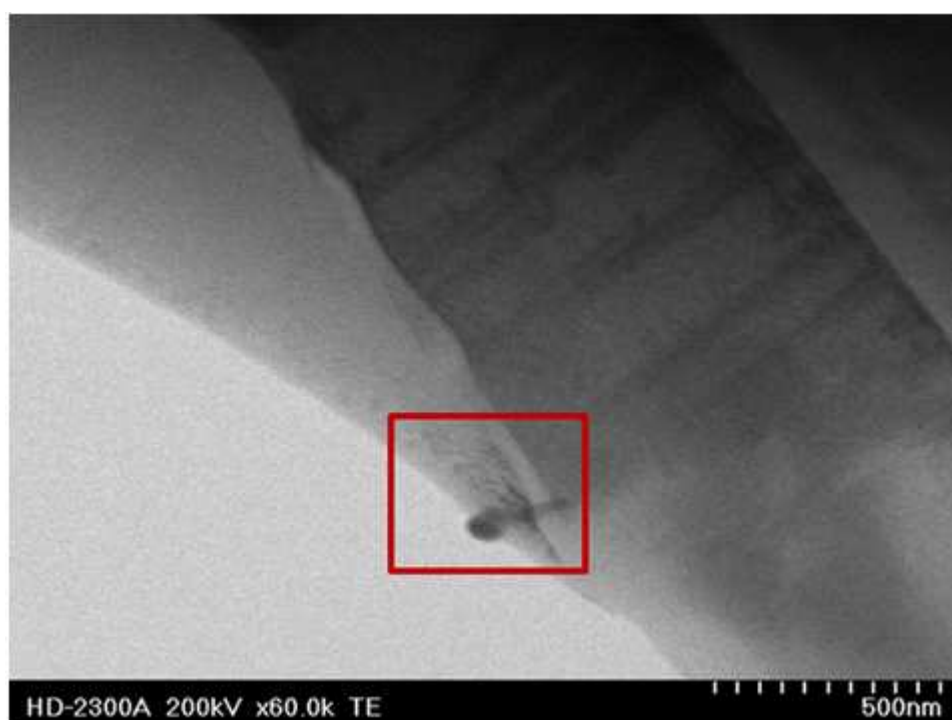
Figure 46 – BF-image from hc wrought alloy (hip 004). Carbide between two grains. Red rectangle indicates location for EDX and EELS measurement.
