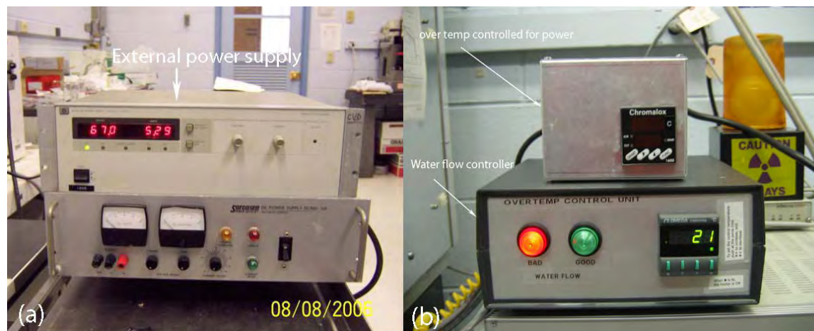
Figure 27. Custom addition to the CSEM tribometer (a) External floating power (b) Custom lab built over temperatures controllers.
