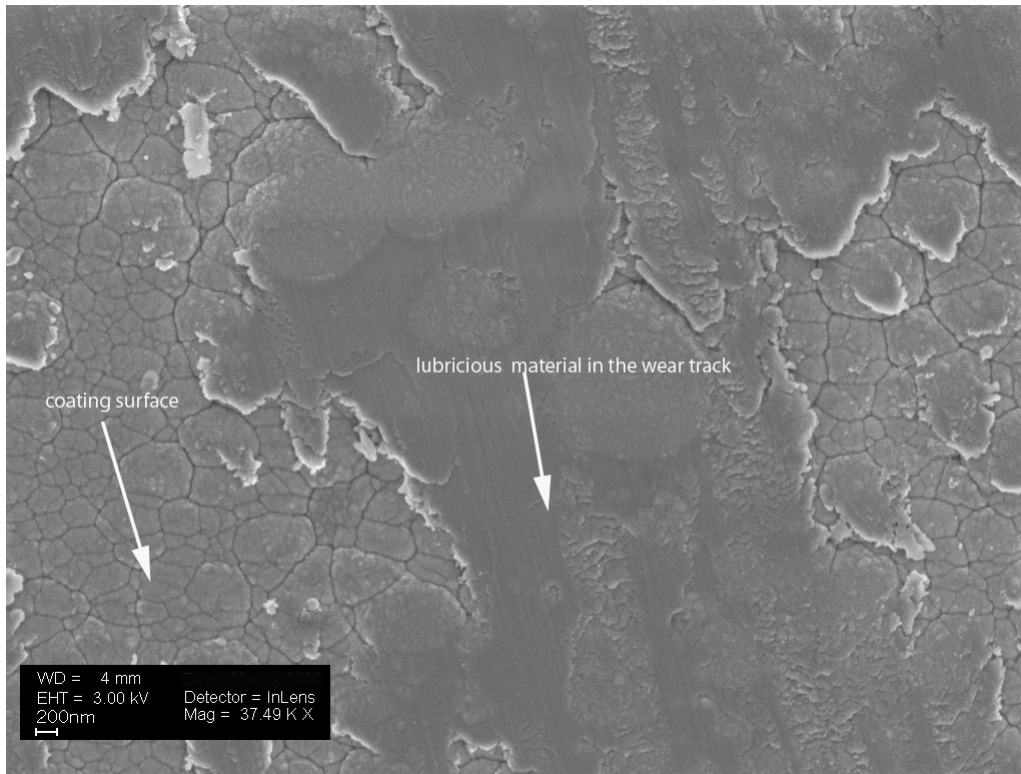
Figure 65. SEM image of the smeared in lubricating soft-phase in the wear track.
