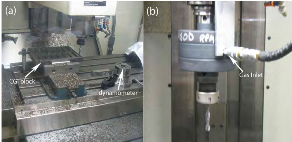
Figure 28. (a) CNC machine at Ford (b) custom made spindle to feed in nitrogen.
