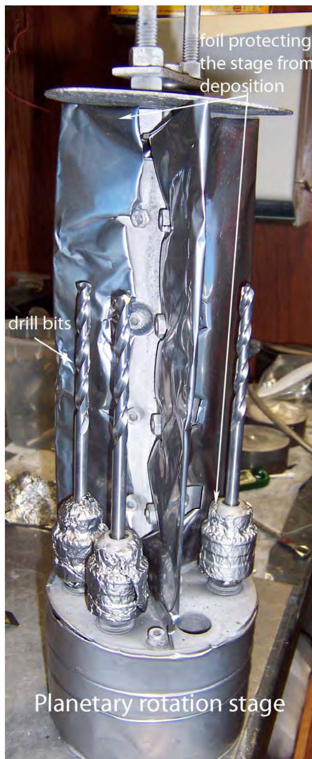
Figure 68. Planetary rotation stage for coating drill bits
