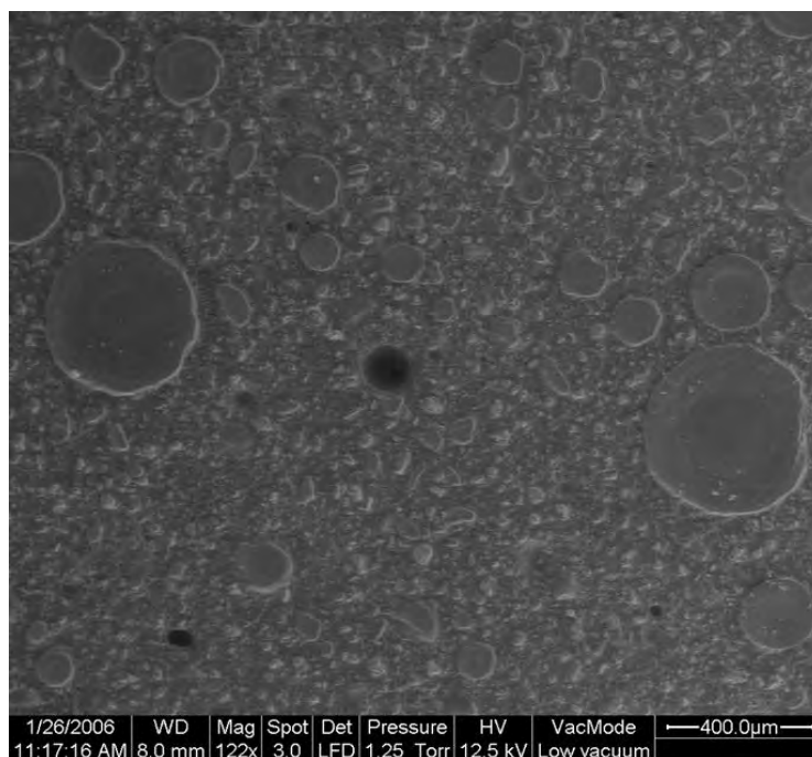
Figure 7.2. Scanning Electron Microscopy Image of Paste with 15% Densified Silica Fume Powder
