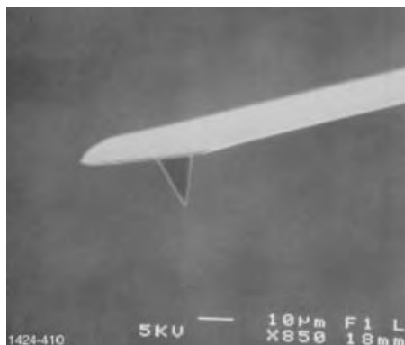
Figure 4.4. Silicon Tip Used in Contact Mode
