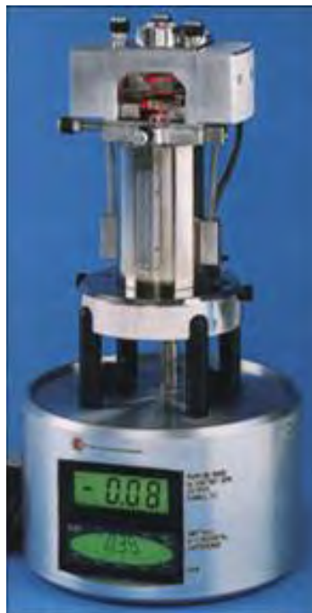
Figure 4.7. Digital Instrument Nanoscope MultiMode Scanning Probe Microscope
