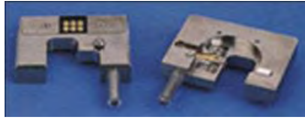
Figure 4.8. Digital Instrument Nanoscope MultiMode Scanning Probe Microscope Tip Holder
