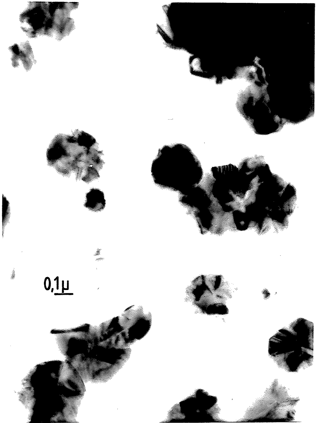
Figure 7.5 Evidence for inter-particle coalescence. This micrograph was obtained through a relatively thin region of the \alpha -alumina support.
