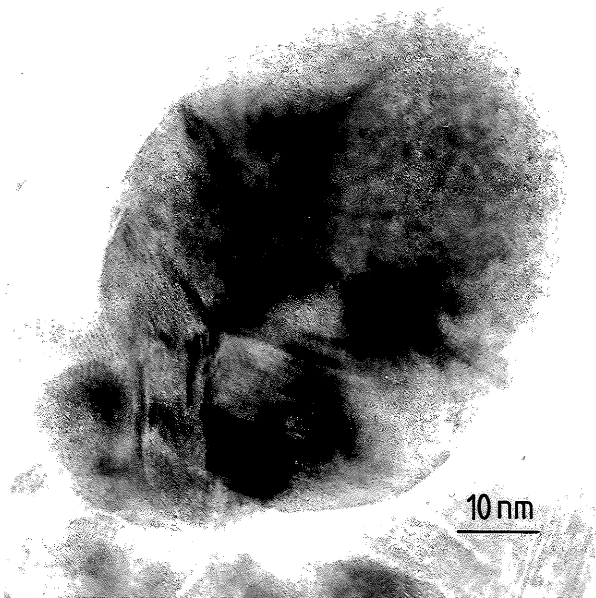
Figure 7.4 High resolution micrograph of a catalyst polyparticle ( taken on the Cambridge H.R.E.M. at 500 kV ). A Dh near to the 5-fold symmetry orientation is present on the lower left, as is shown by the lattice fringe configuration.
