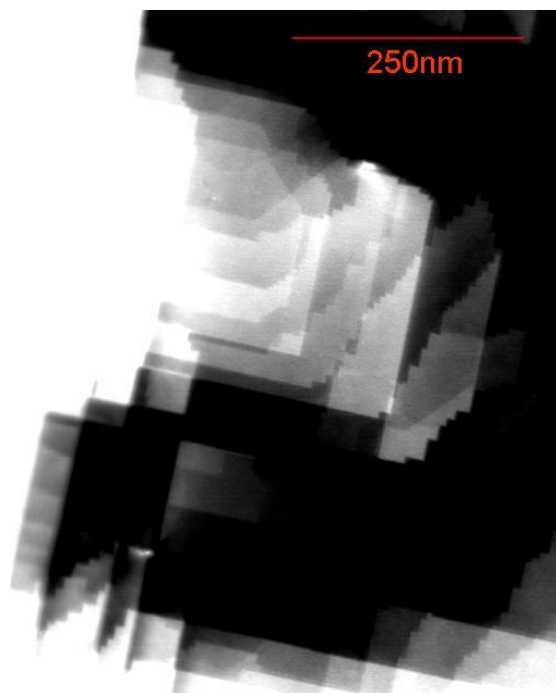
Figure 4.1. Dark field TEM image showing surface faceting along \langle 010 \rangle and \langle 100 \rangle directions and reconstructed step surfaces.
