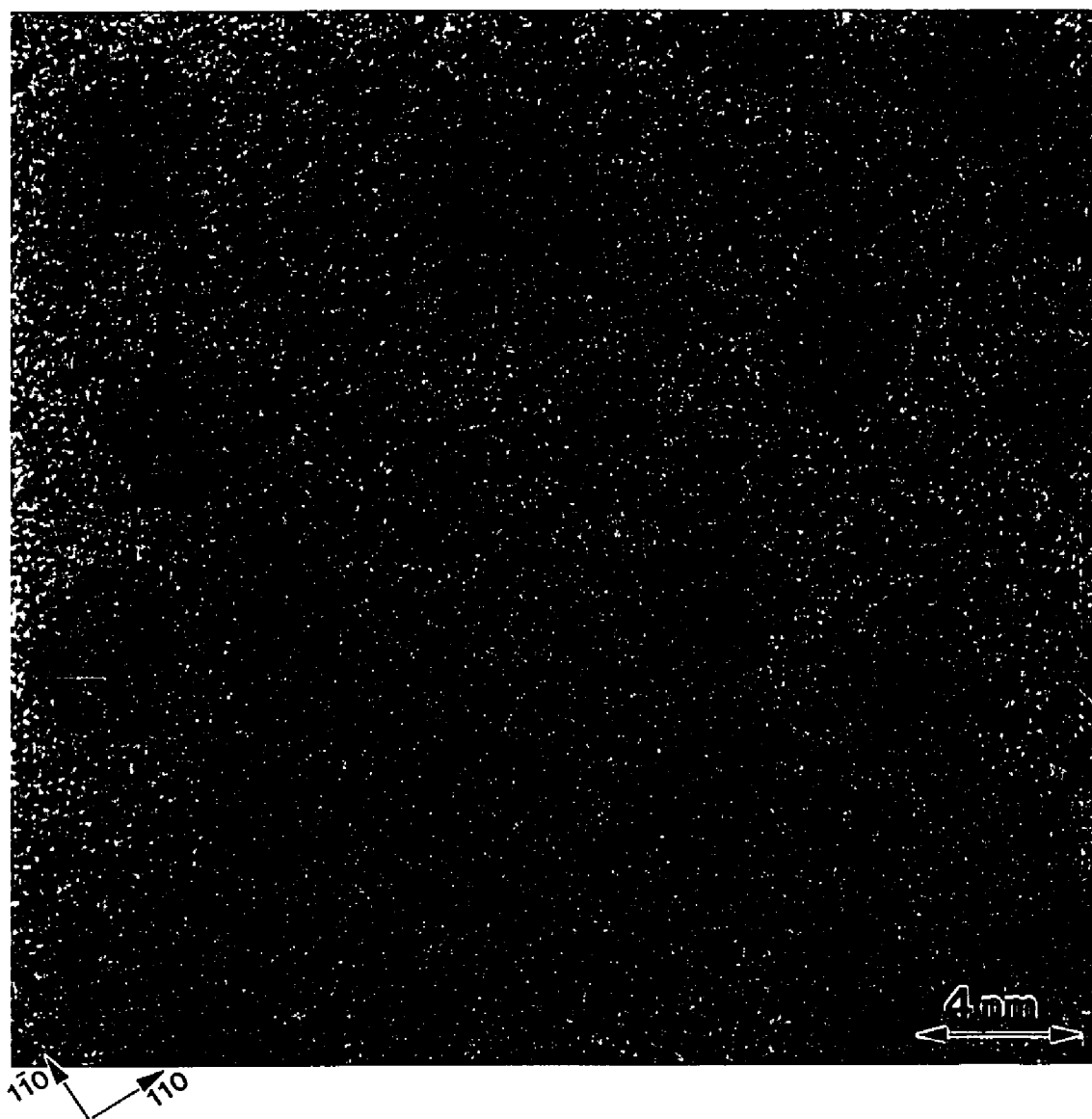
Figure 4.4. An off-zone image of the Ag-Si(001)-2x1 interface. The features with the moiré fringes in Figure 4.3 are resolved to be three-dimensional islands of Ag.
