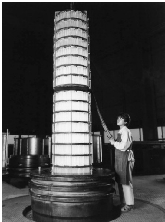
Figure 2.2. Illustration of scale of autoclave used to grow large single crystal of quartz, of several meters in length. Figure adapted from reference [35].
