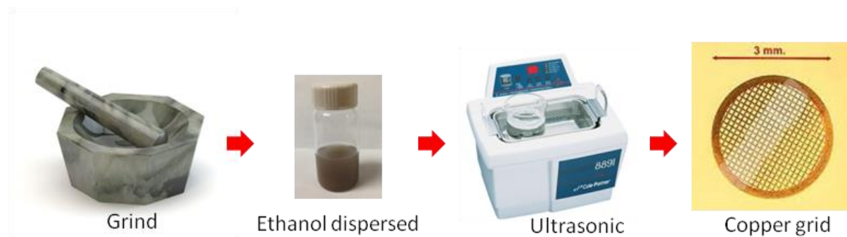
Figure 2.1. Schematic diagram shows the procedure for Pt/STO-NCs TEM sample preparation on copper TEM grids.
