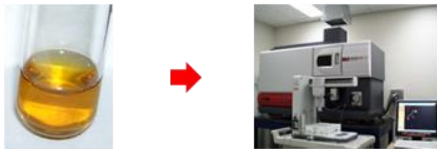
Figure 4.3. A light yellow solution of 5 mg Pt/STO dissolved in a mixture of 1 mL of nitric acid with 3 mL of hydrochloric acid.
