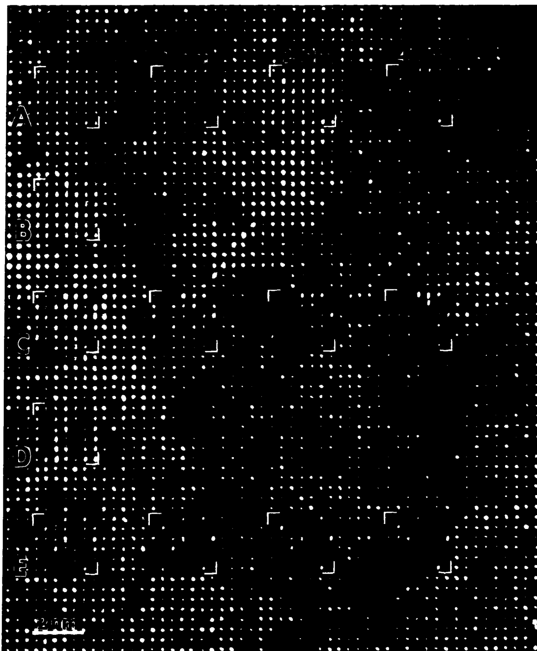
Figure 3.7 HREM image (214 nm underfocus) down the \langle 001 \rangle zone axis with simulations of defect models A-E inserted. Models A, C, and E have amorphous carbon added to the top and bottom surfaces as explained in the caption for Fig. 3.5. Note that with increasing amorphous carbon there is an increasingly evident periodic dark contrast not seen in the experimental image.
