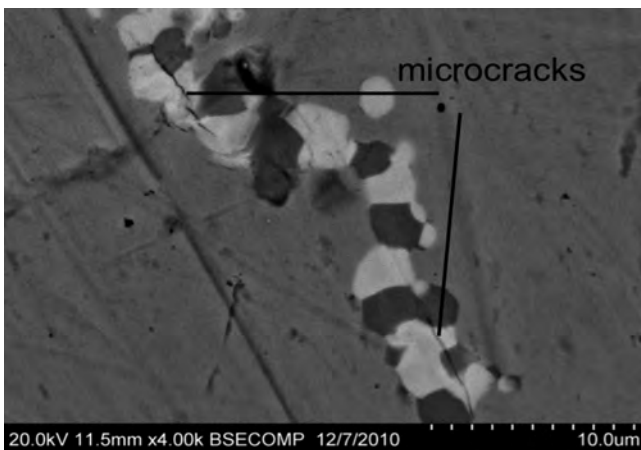
FIG. 8—Microcracks within IPs (lighter phase) within the primary articulating area of retrieval 2.
