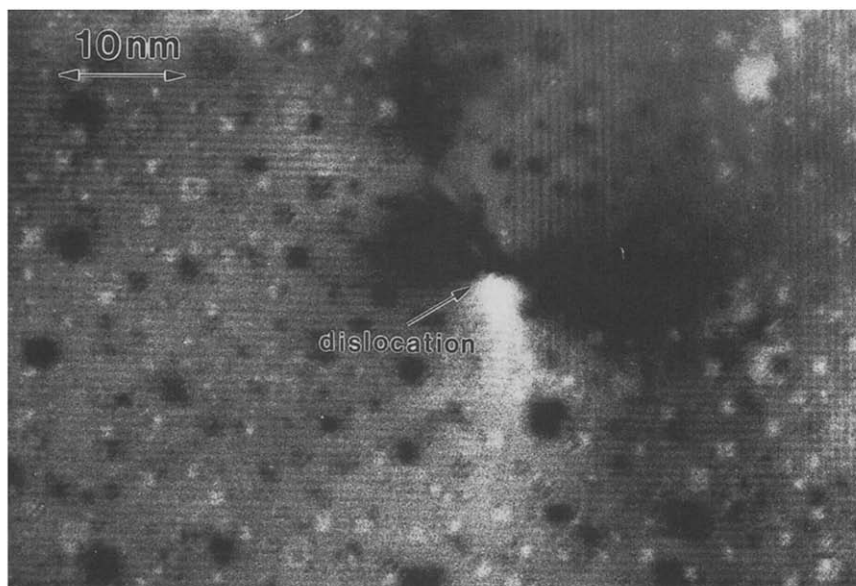
Fig. 6. Dark field micrograph showing a dislocation coexisting with the reconstruction. The reconstruction does not seem to be disturbed by the strain field of the dislocation, since moiré fringes are seen to run straight past the dislocation.
