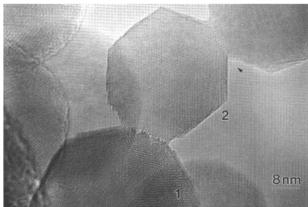
FIG. 6. Chain of sintered particles where the neck regions can be considered as atomically irregular. The middle particle (#2) has a distorted shape (arrowed) with respect to the Wulff construction as a result of the sintering process. Furthermore, the {220} facet of particle 1 is sintered to the {111} facet of particle 2, giving an atomically irregular interface.
