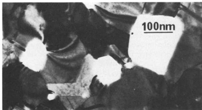
Fig. 1. Low magnification image showing the typical morphology of the semi-continuous, holey Au films.
