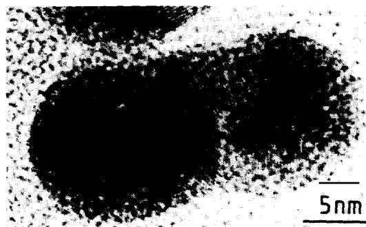
Fig. 10. Example of a decahedral MTP forming a bridge between two icosahedral MTPs.
