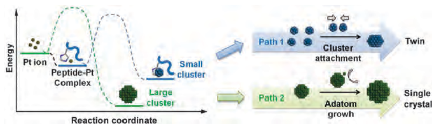
Fig. 19 Growth pathways for metal nanocrystals mediated by peptides: cluster attachment (Path 1) or adatom growth (Path 2). Cluster attachment is more likely when the precursor–ligand complex is specifically stabilized, such as by interactions between histidine and \text{Pt}^{2+} ions, that lead to an increase in activation barrier, smaller clusters, and twin crystal formation (Path 1). Adatom deposition is faster in the absence of significant precursor stabilization, which leads to larger clusters, and single crystal formation (Path 2). Reproduced with permission from ref. 110.
